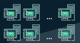
Workstations and GPUs in the traditional deployment model are configured on a 1:1 basis, having a dedicated GPU installed, and depending on chassis size, a limited number of supported GPUs. Additionally, power requirements and heat generation must be considered.
